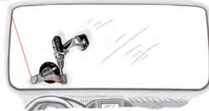
Upon reaching the top right corner, change the position again to the top left corner (Fig. 5). Then change position to the bottom left corner (Fig. 6) and complete the removal process.
