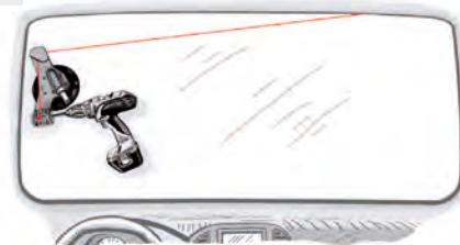
Use the cordless screw driver slowly to the right, adjusting the speed depending on load. During this process hold the removal protector internally between the windscreens removal cord and the dashboard, shaft or roof lining, so that the interior of the vehicle cannot be damaged. Now continue with the removal process until the windscreens removal cord has reached the bottom right corner .
