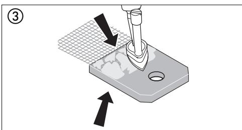
③ On one side, fuse the stainless-steel mesh into the plastic. Heat the mesh all over and fuse by applying even pressure.
