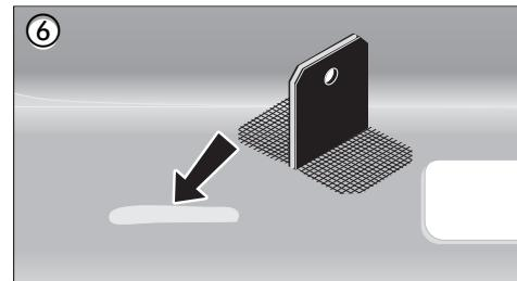
⑥ Position the tab at the intended position and fuse both sides into the bumper plastic using the vehicle repair nozzle. For better results at the tab base, the tab can be bent slightly towards the other side.
