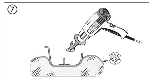
⑦ **TIP:** With this method of tab attachment, it is recommended to place damp cloths or a cold jelly pad underneath to avoid deformation.
