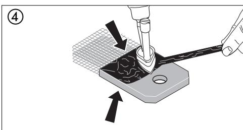
④ Using the plastic repair nozzle, carefully apply the Multi-Thermoflexx welding rod. Rod and surface must be evenly heated and completely bond with the surface. Slowly smoothen the material at the edges. Using the plastic repair nozzle, fuse the stainless steel mesh into the plastic on the rear of the tab. Now apply the Multi-Thermoflexx welding rod and carefully fuse with surface.
