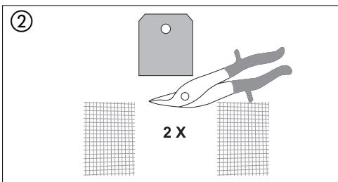
② Cut stainless-steel mesh to tab width for both sides of the tab. Length approx. 60 mm, half-projecting.
