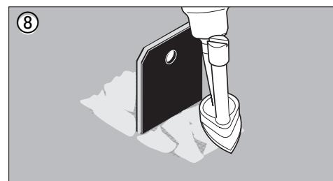
⑧ – ⑩ Apply the Multi-Thermoflexx welding rod and slowly and carefully smoothen the material at the edges.
