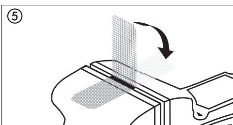
⑤ Bend apart the projecting mesh at an angle of 90°.
