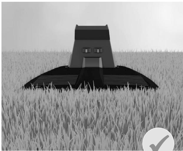
**EN:** Make sure the docking station is placed on level ground. This will allow the Indego to dock correctly.
